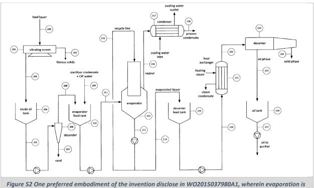
Figure 52 One preferred embodiment of the invention disclose in WO2015037980A1, wherein evaporation is carried out prior to separation using a two- phase decanting centrifuge and evaporation achieves substantially complete removal of the free water..
