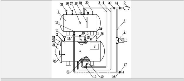
Figure 6 A semi-automatic double-layer hot water circulating oil palm fruit sterilizing tank as disclosed in CN203498354
