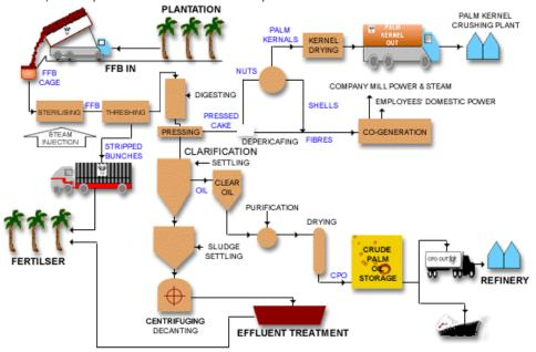
Figure 2 Crude palm oil milling process (Source: <u>http://www.oilrefineryplant.com/palm-oil-processing</u>)
