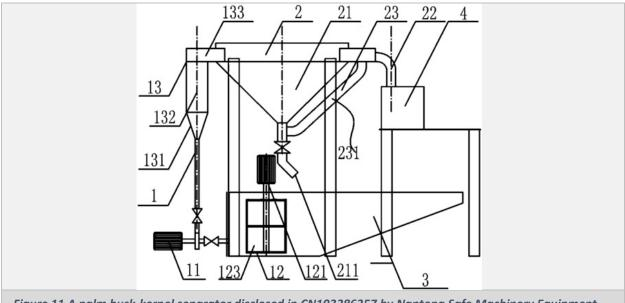
Figure 11 A palm husk-kernel separator disclosed in CN103386357 by Nantong Safe Machinery Equipment.
